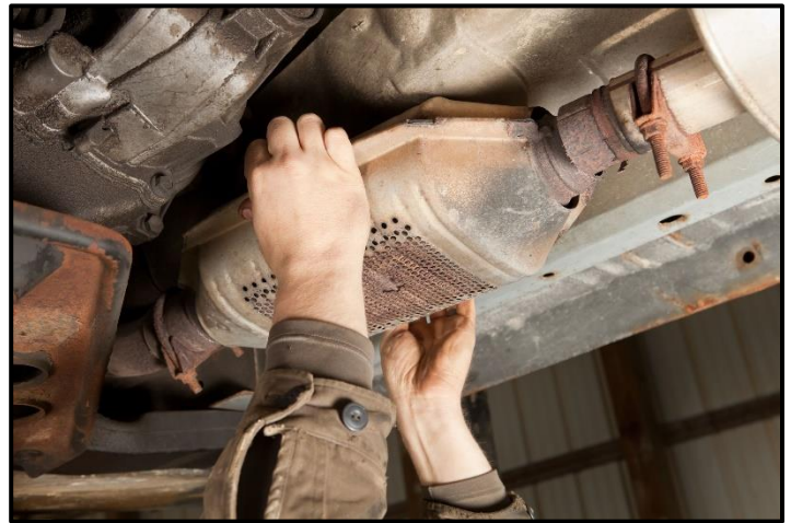
EASY-PEASY: Catalytic converters can be removed from a vehicle in only a few minutes.
